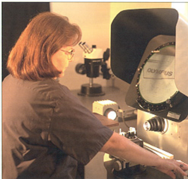
ENGINEERING IT IN: Screen Tech's quality auditor Sharon Robertson views a graphic design element on the optical comparator, one of a number of QC tools available to her in the company's Quality Assurance Department. Job one? Maintain Screen Tech's ISO 9000-level quality process.
