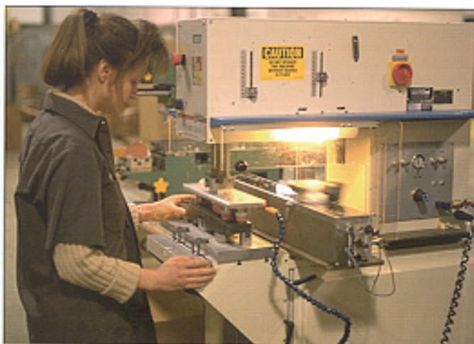
NOT FLAT? NO PROBLEM: Pad-transfer equipment extends the Saddlers' printing capability to keypad buttons and other irregular or hard-to-reach plastic surfaces on their client's injection-molded parts.
