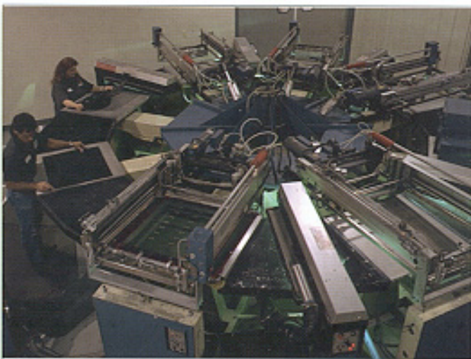
INLINE AUTOMATION: Screen Tech's Hercules 5-color, carousel UV screen printer is the centerpiece of the Saddler's screen-printing department, the most efficient tool in a process-quality arsenal that includes an additional half-dozen semi- and three-quarter-automated presses.
